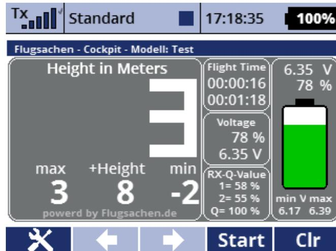
In the large window on the left, the altitude data is displayed as values or as an instrument, depending on the setting used. The height gain (+height) can be set to zero using the switch.
