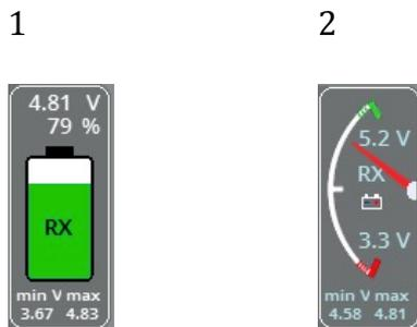
The displayed voltage depends on the selected sensor and the set values. The selected sensor is shown in the display, RX = receiver battery, S1 and S2 for sensors e.g. Jeti CB Box. The displayed values are set in the third window, Battery.
