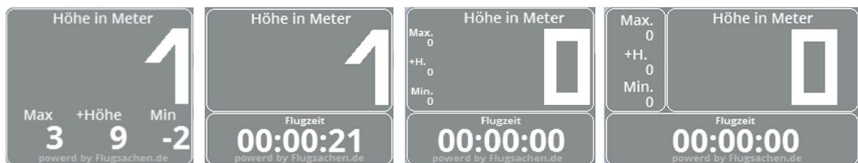
Display 1 shows the current altitude in large digits at the top and the maximum altitude, altitude gain and minimum altitude below.
